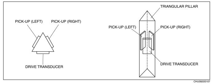
• One face of the triangular pillar functions as the driving side, the others function as pick-up sides. Electrically induced vibration of the drive transducer causes the pick-up sides to vibrate, and the pick-up sides produce an electrical current.
