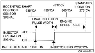
The injection end position is determined by the engine speed. (The higher the engine speed the lower the fuel injection timing.)
