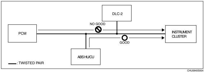
3. If there is a communication error between the ABS HU/CM and PCM, or between the instrument cluster and PCM, even if the communication between the ABS HU/CM and the instrument cluster is normal, it is probable that there is a malfunction in the PCM or PCM-related wiring harnesses.
