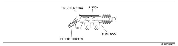
• Due to spring pressure maintaining play between the push rod end and the release fork at zero, an automatic adjusting, maintenance-free design has been achieved.
