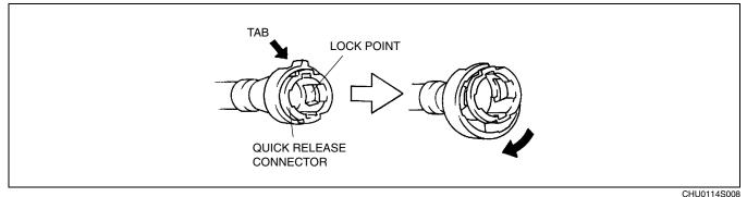
• To connect the quick release connector properly, push it into the fuel pipe until a locking click sound is heard.
