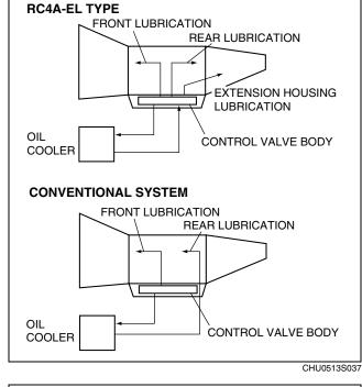
• A passage located in the rear of the extension housing supplies a steady amount of lubricant exclusively to the bushing.
