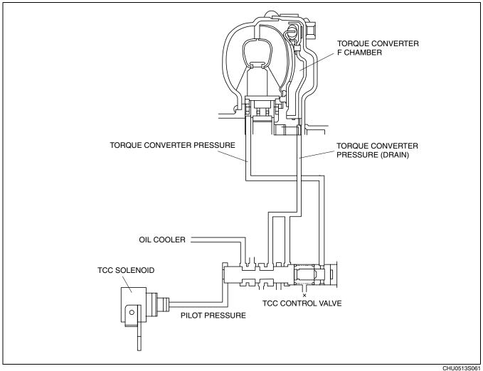
**Determination of TCC inhibition**
