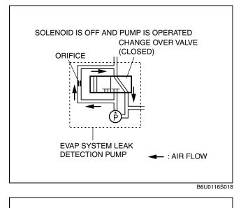
• Air taken from the air filter is sent to the charcoal canister via the pump.
