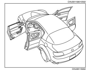
• The rear doors have been slanted towards the inner side and rear of the vehicle so they open at a slightly upward angle. This prevents the doors from interfering with each other when opening or closing and reduces the amount of force required for opening.
