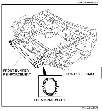
A three-pronged structure, capable of dispersing impact force received by the front side frame in three directions, has been adopted. It also suppresses cabin deformation in offset frontal collisions.
