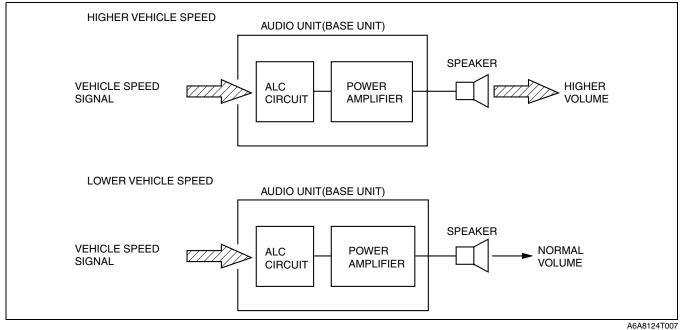
• The ALC function is divided into four modes, and can be used effectively to match the driving conditions.
