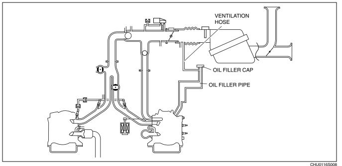
**POSITIVE CRANKCASE VENTILATION (PCV) VALVE OPERATION**
