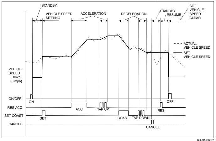
• The cruise control includes the cruise control operation condition and the cruise control stop condition.
