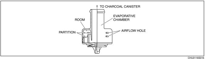
• A small section with partitions is located in the evaporative chamber. These partitions protect the charcoal canister by preventing flooding as atmospheric air enters from the airflow holes.
