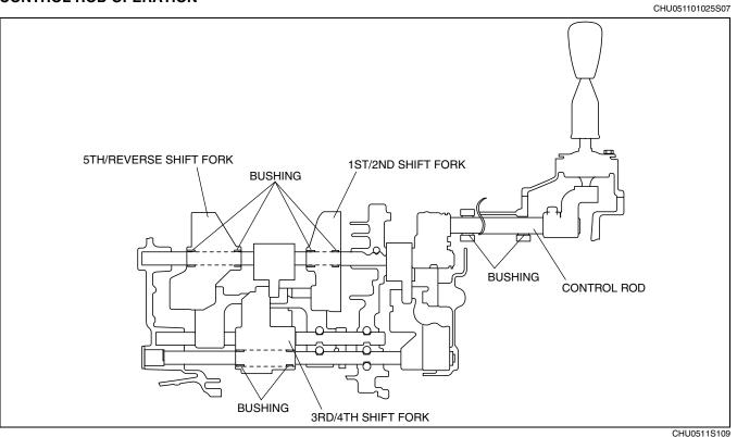
• The control rod sliding section and the supports of each shift fork are equipped with a teflon bushing, which reduces sliding resistance during shifts and thus improves shift feeling.
