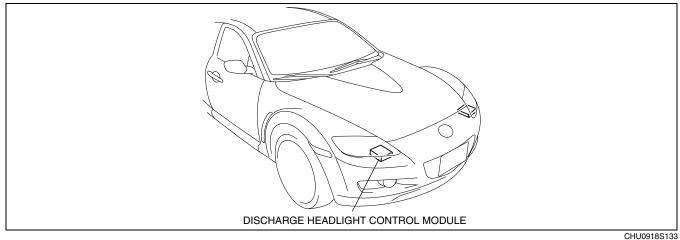
• Switches the direct current from the battery to alternating current (25,000 V) and optimally controls the current supply output to the bulb.
