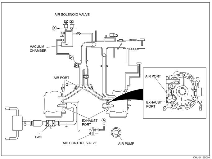
SECONDARY AIR INJECTION (AIR) CONTROL VALVE FUNCTION
